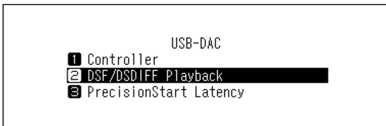
6 Select the playback mode for supported DSD files and press the
